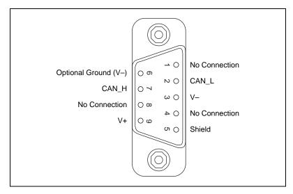
Figure C-1. Pinout for 9-Pin D-Sub Connector
